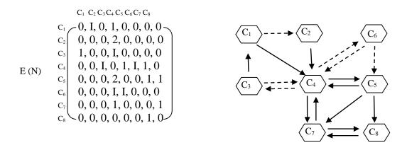
The combined overlap block connection matrix of FCM is given by E.
