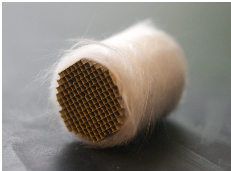
Figure 14. A coated substrate (2SSC) is wrapped in quartz wool in preparation for testing.
