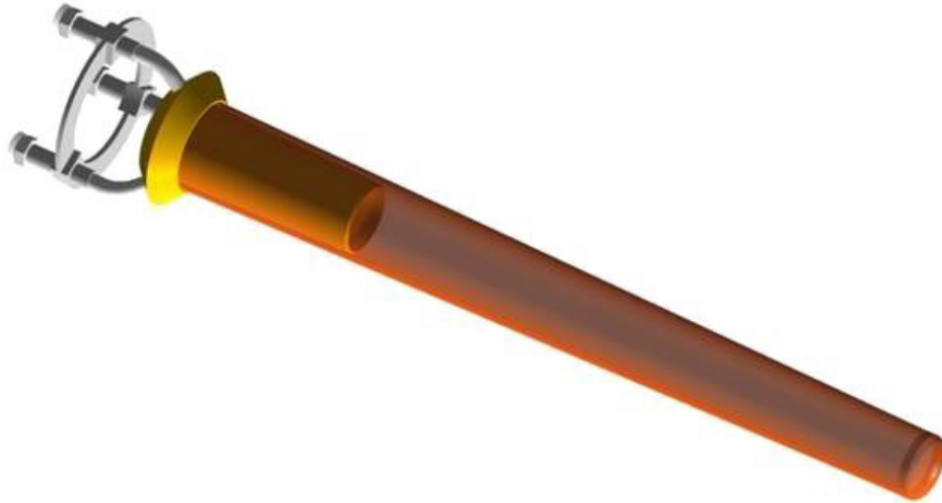
FIG. 12: A schematic of the target inside the CLAS detector.
