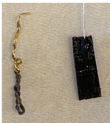
Figure 20. Fabricated Au-co-Pt anode on left and GDE cathode on the right.
