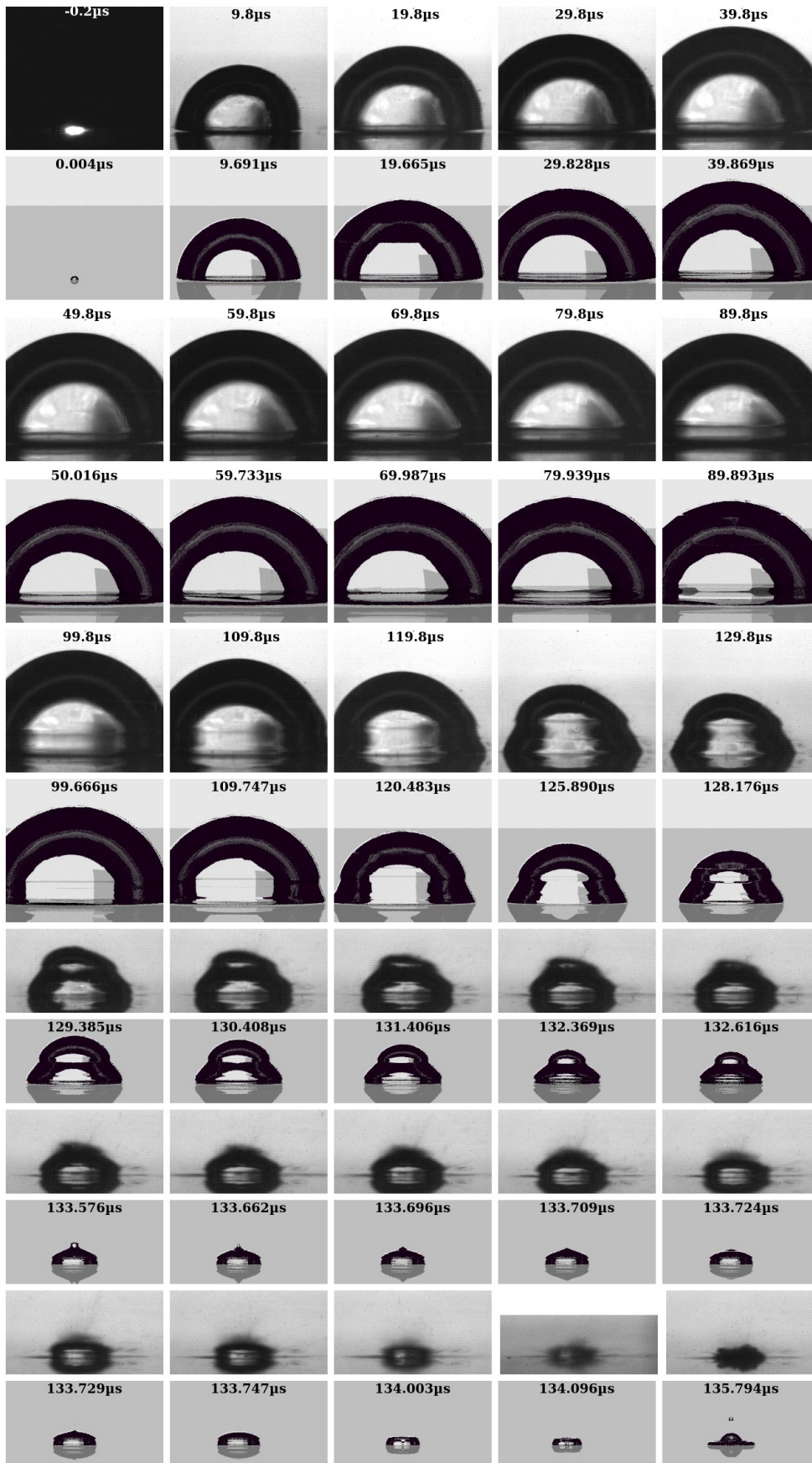
Fig. 5.2: Overlay of the simulation of Fig. 5.1 (even rows) and experimental recordings (odd rows) using setup 1 (Sec. 3.3.1) for a D^* = 0 bubble. The experimental images with a time annotation belong to the same measurement, the remaining 16 experimental frames are from 15 different measurements. Frame width is 1048 \mu\text{m} .
