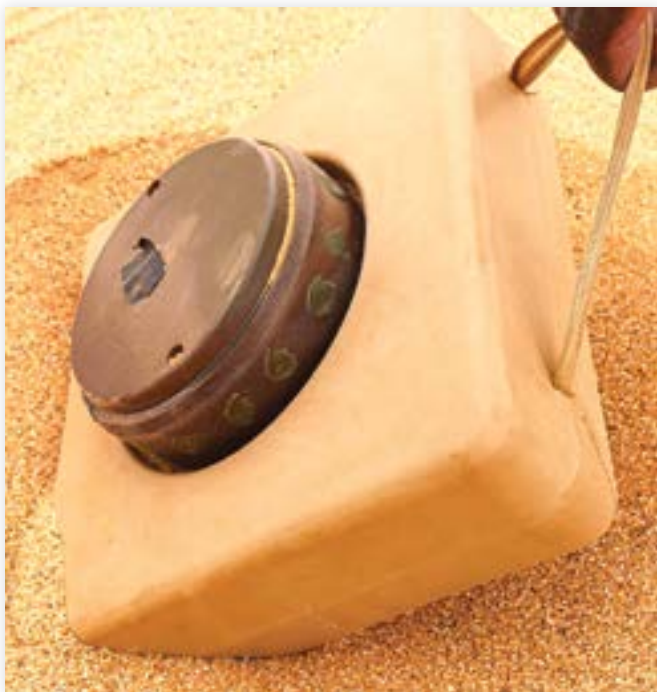
Image 4. The PRB-M3A1 landmine, which showed different thermal anomaly characteristics from the pressure plate than the square plastic body filled with 6 kilograms of explosives.
