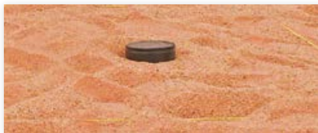
Image 5. Our reference PMA-3 anti-personnel landmine was buried at a depth of 1 cm. It is shown above after excavation at the end of the study. The type of sandy environment can also be seen.
