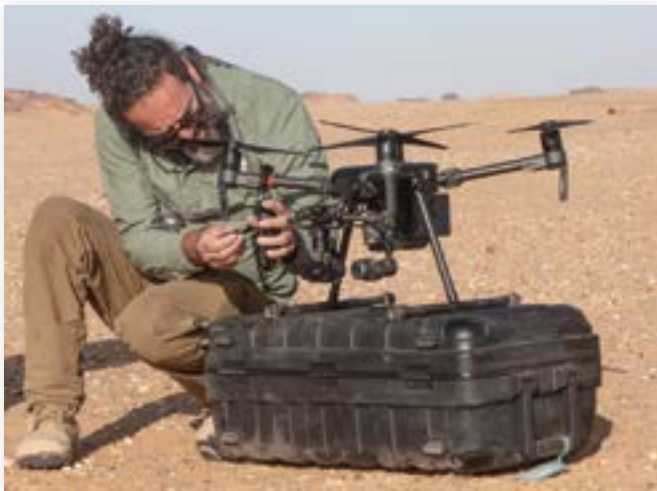
Image 3. Fieldwork at remote, in-situ Sahara Desert minefields using a small industrial model, off-the-shelf, DJI Matrice M210 v2 quadcopter with advanced sensors.
