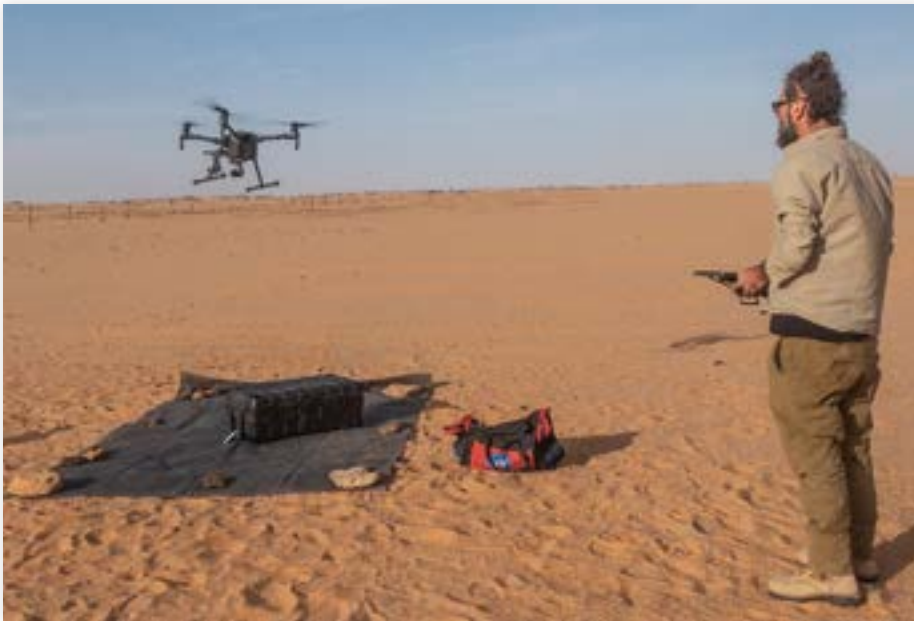
A 2019 upgrade to the system appearing in Figure 2. Here, the author uses small drones to fly thermal/LWIR sensors over legacy desert minefields in Chad. Sadly, real-world thermal/LWIR data has been scarce since 2005.
