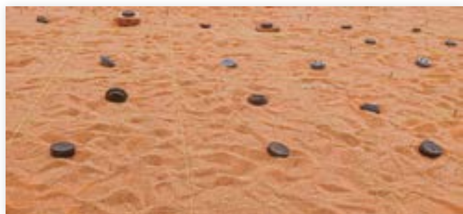
Image 2. Setting up the controlled field test site to bury: production, FFE, and simulant landmines from where IR thermography data was automatically captured at one-minute intervals, 24-hours a day.
