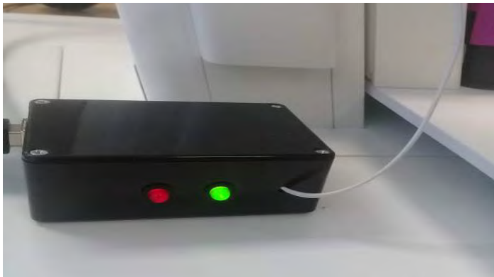
Figure 4: Sensor attached to sit-stand worktables recording sit-stand transitions in the physical condition.
