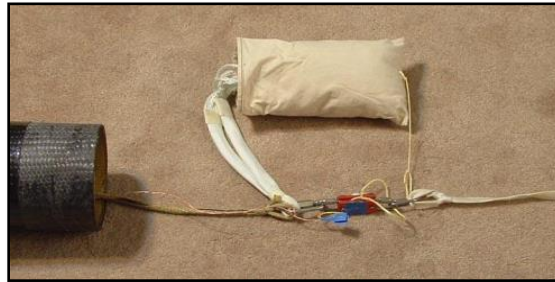
Figure 90 - Tender Descender layout and wiring
