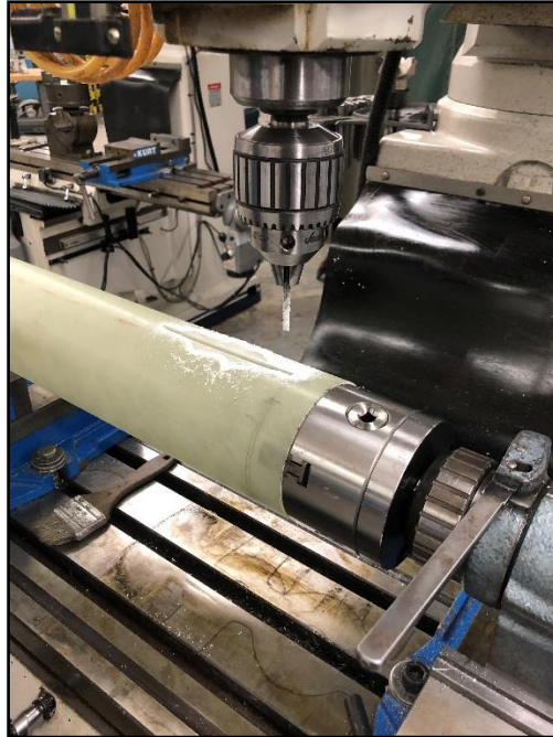
Figure 155 - Subscale booster fin slot manufacturing with an end mill in the machine shop
