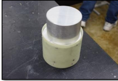
Figure 137 - Shear Test tube setup
