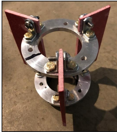
Figure 148 - Subscale assembled fin retention system
