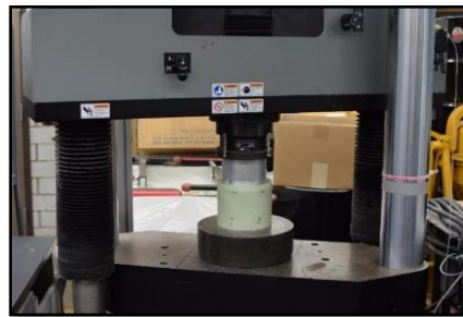
Figure 138 – Fiberglass body tube setup in INSTRON machine before shear test
