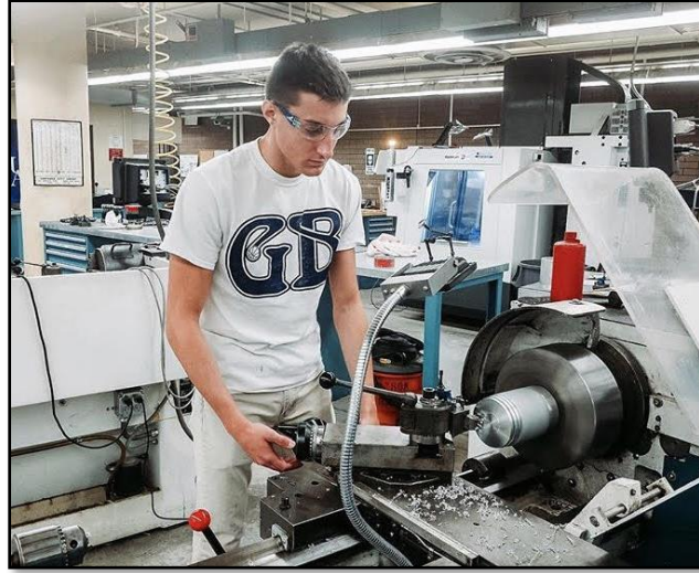
Figure 149 - Senior design team member manufacturing bulkheads with a manual lathe in the machine shop
