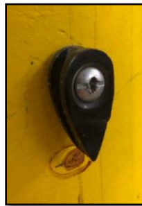
Figure 63 - Commercial rail button mounted to airframe
