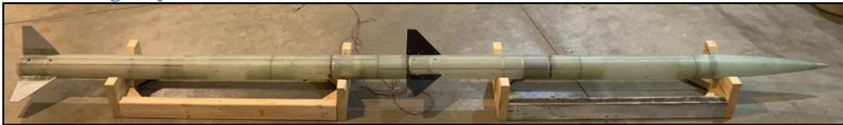
Figure 153 - Subscale rocket airframe layout
