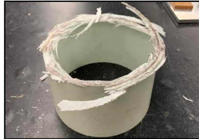
Figure 135 - Compressed tube in INSTRON machine post-test
