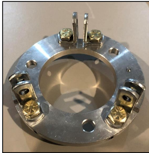
Figure 147 - Subscale assembled centering ring for fin retention
