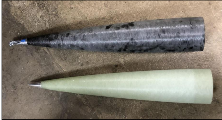
Figure 6 - 5:1 (top) and 5.5:1 (bottom) fiberglass Von Karman nose cones
