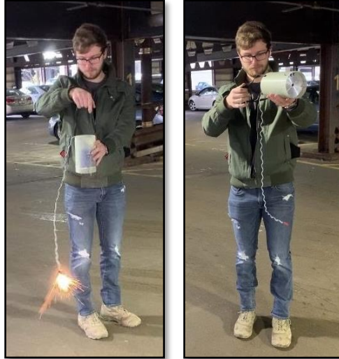
Figure 144 - EasyMega angle testing within 20-degrees (left) and outside of 20-degrees (right)
