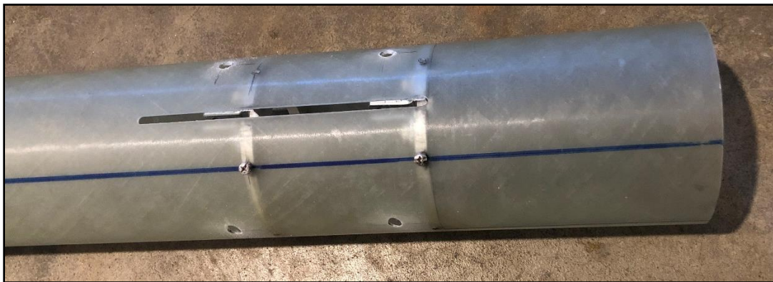
Figure 154 - Subscale sustainer fin slots with assembled centering rings
