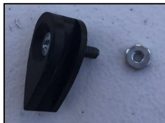
Figure 64 - Rail Button Hex Nut attachment method
