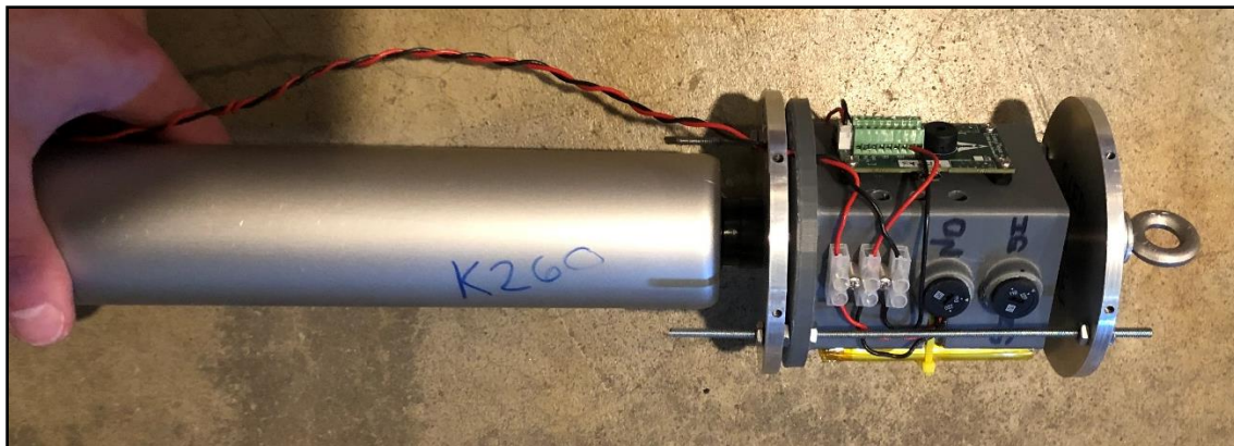
Figure 151 - Subscale sustainer motor retention with eyebolt
