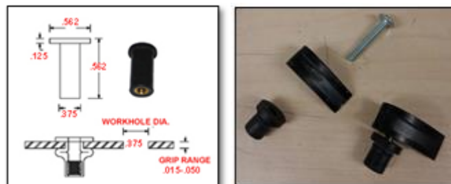
Figure 65 - Rail Button Threaded Insert
