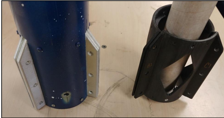
Figure 44 - Akronauts' previous 3D printed fin retention canisters
