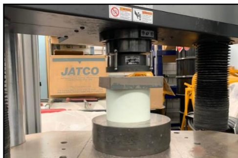
Figure 134 - Fiberglass body tube setup in INSTRON machine before compression test
