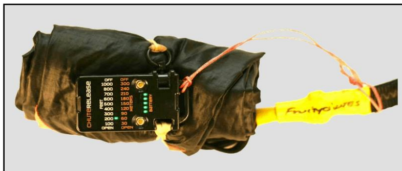
Figure 91 - Jolly Logic chute release assembled to a parachute
