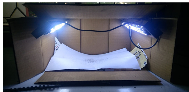
Fig. 2 Laboratory set-up for image acquisition of coal samples
