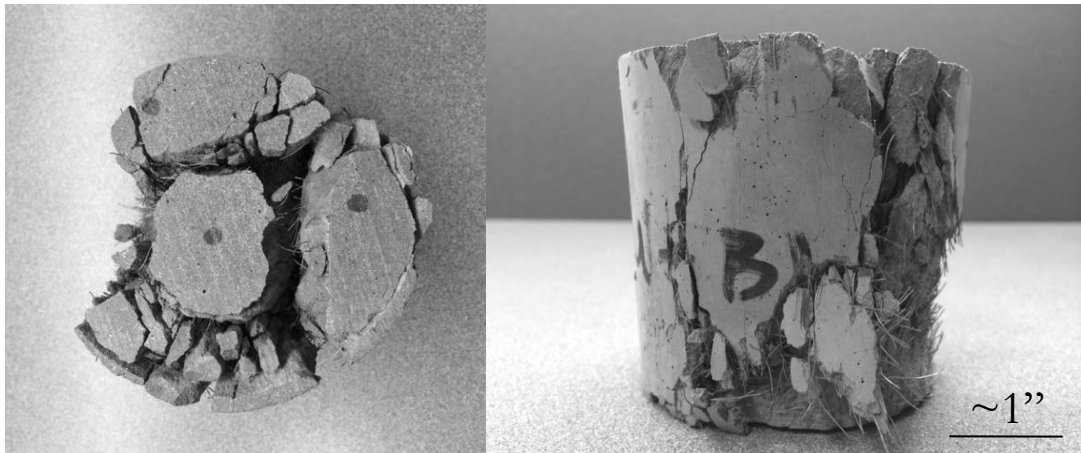
Figure 5.4: Typical fracture of UHPC at 1:1 aspect ratio
