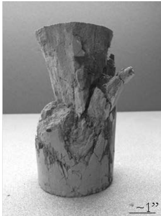
Figure 5.3: Typical fracture for UHPC at 2:1 aspect ratio
