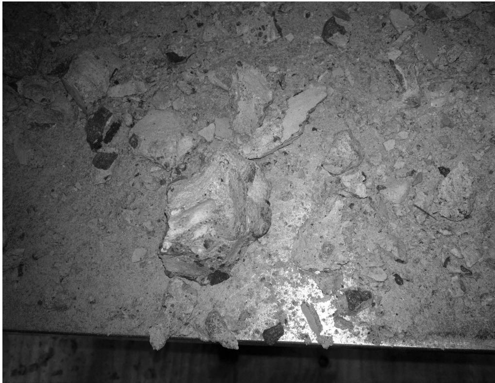
Figure 5.1: Typical NSC fragmentation following SHPB test
