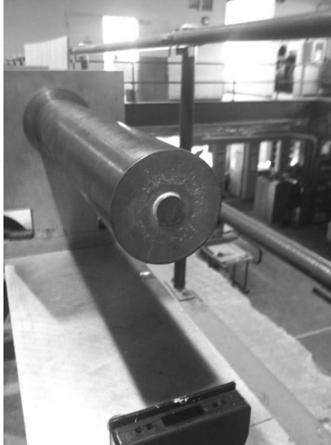
Figure 3.6: Copper pulse shaper placed on impact face of input bar
