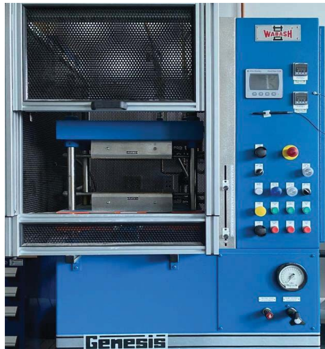
Figure 2.2 Wabash hot-press used to cast the sample.
