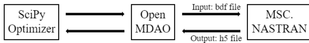
Figure 5.11 File interaction between OpenMDAO/SciPy and MSC. NASTRAN.
