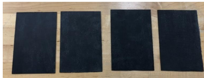
Figure 3.3 Trimmed composite samples for LVI testing (total is 6).
