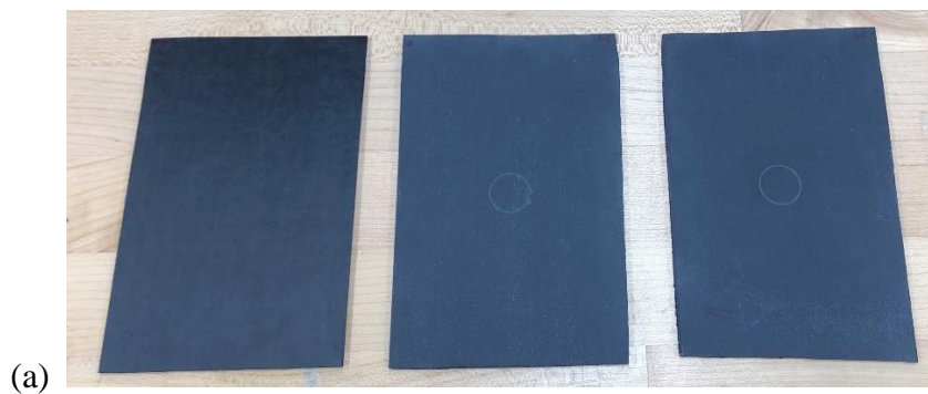
Figure 3.6 Impacted plates with hemispheric tip impactor, a) front side, and b) backside, from left to the right: 1 m/s, 1.5 m/s, and 2 m/s.
