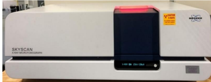
Figure 3.8 Skyscan X-Ray Microtomography (15 kv, 150 \mu A).
