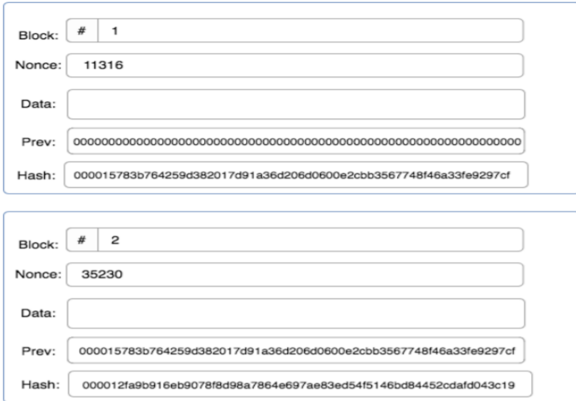
Figure 5. Two blocks are chained together to form a blockchain.
