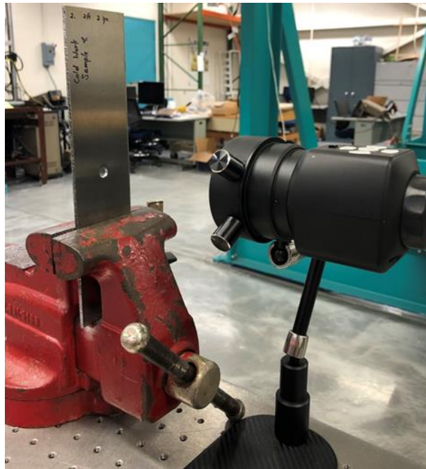
Figure 3.9 Experimental apparatus of speckled sample and UHM350-11 digital microscope to map strain development during the cold expansion process.
