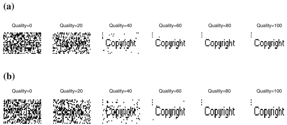
Fig. 7 Extracted watermarks under JPEG Compression attack with different quality factors. a DWT–FRFT watermarking method. b Proposed FWT watermarking method
