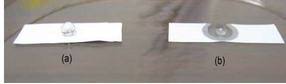
Fig 5-1. Wettability test of (a) hydrophobic ePTFE, and (b) hydrophilic ePTFE
