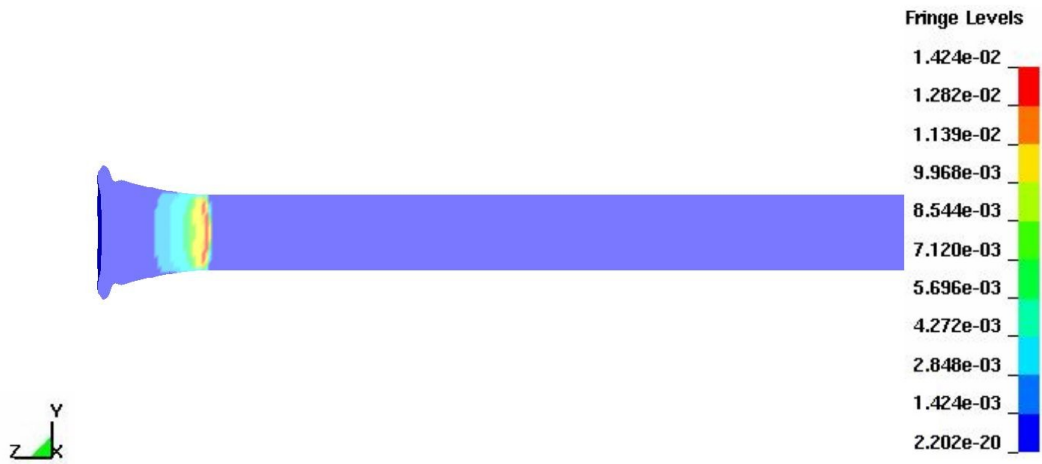
Figure 5.18: Reacted material characterization simulation, pressure contours at time = 19.40 \mu\text{s} .
