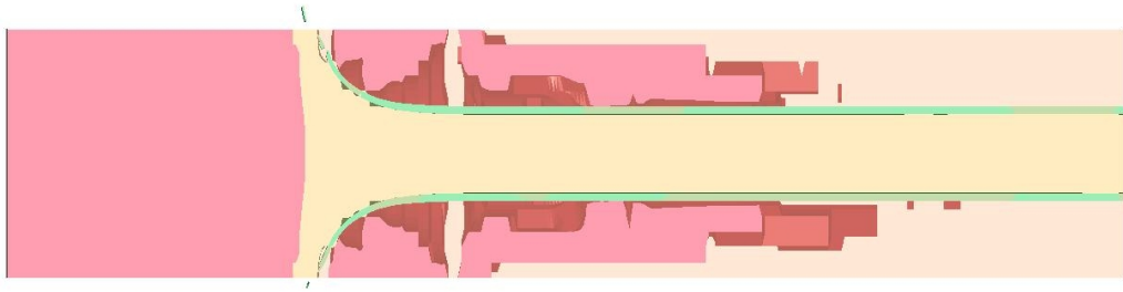
Figure 5.12: Reacted material characterization simulation, material locations at time = 116.4 \mu\text{s} .
