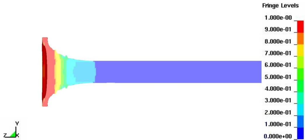
Figure 5.32: Reacted material characterization simulation, percent reacted at time = 77.60 \mu\text{s} .
