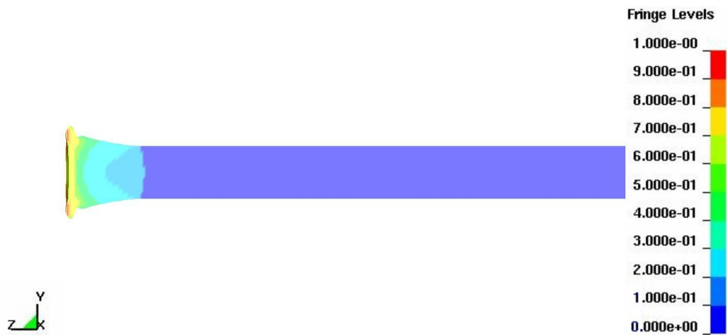
Figure 5.29: Reacted material characterization simulation, percent reacted at time = 19.40 \mu\text{s} .
