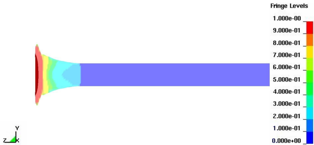
Figure 5.30: Reacted material characterization simulation, percent reacted at time = 38.80 \mu\text{s} .
