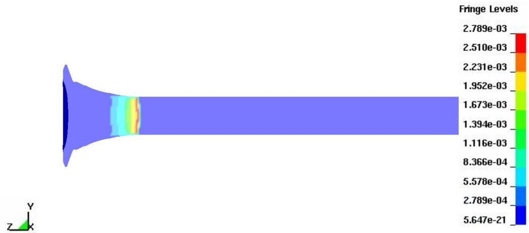
Figure 5.19: Reacted material characterization simulation, pressure contours at time = 38.80 \mu\text{s} .
