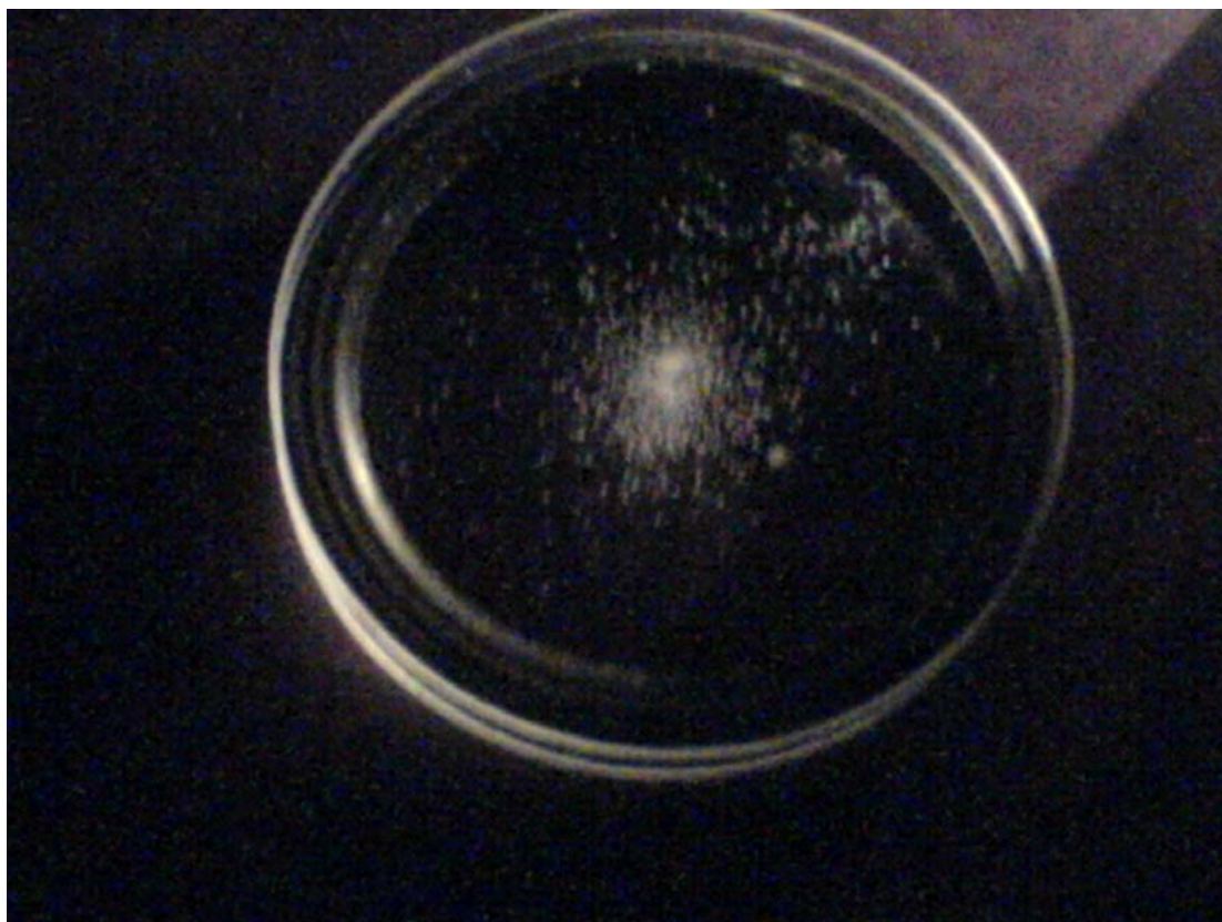
Fig. A1. Photograph of 38 mm diameter fused silica window resting on an o-ring. The white photochemical product is apparent.
