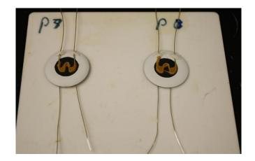
Fig. 10: Fuel cells with silver wire test leads in M-shape configuration
