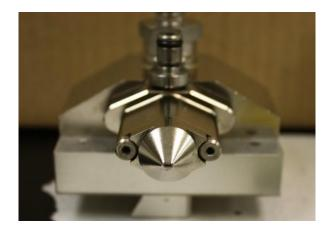
Fig. 7: Deposition nozzle head of the Optomec AJDT system
