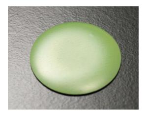
Fig. 5: Bisque-fired anode substrate
