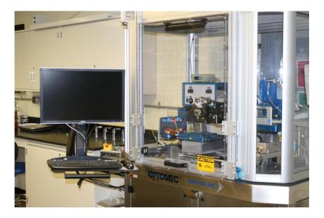
Fig. 3: Optomec Aerosol Deposition System
