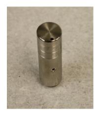
Fig. 8: Atomizer within the Optomec AJDT system
