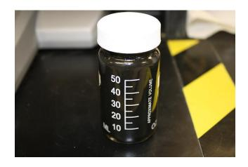
Fig. 6: Prepared LSCF ink within a wheaton bottle container
