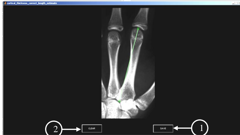
Figure 4.6: GUI to manually adjust the approximate length. The user clicks on the most distal end of the metacarpal and then drags the mouse to the most proximal end of the metacarpal to draw the approximate length line. Once the user is satisfied with the manually adjusted approximate length line, pressing (1) the ‘SAVE’ button updates the values and returns the user to the main GUI. (2) The ‘CLEAR’ button deletes the manually drawn line.
