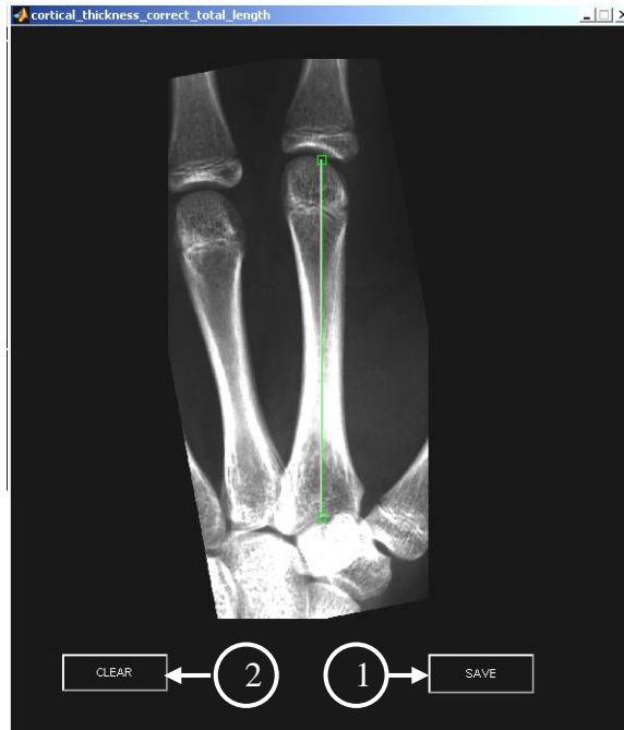
Figure 4.7 : GUI to manually adjust the total length. The auto generated line is initially displayed along the long axis of the metacarpal (since it is difficult for the user to position the line along the exact bone midline), and the user simply adjusts the endpoints of this line as needed. Once satisfied with the manual adjustment, pressing (1) the ‘SAVE’ button updates the values and returns the user to the main GUI. The user also has the option to clear the total length line by selecting (2) the ‘CLEAR’ button.
