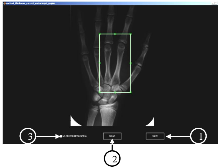
Figure 4.4: GUI for manual metacarpal ROI selection. A rubberband box is drawn around the metacarpal of interest and the medially adjacent metacarpal. This box may be deleted by pressing the (2) 'CLEAR' button. Once the user is satisfied with the selected ROI, pressing the (1) 'SAVE' button stores the ROI coordinates, and returns control to the main GUI. If the metacarpal of interest is not present in the image, the user presses the (3) 'NO METACARPAL' button and then presses (1) 'SAVE' to exit this GUI.
