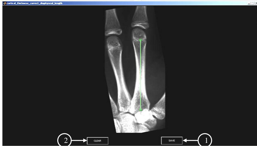
Figure 4.8: GUI to manually adjust the diaphyseal length. (1) As with the total length, the auto generated line is initially displayed along the long axis of the metacarpal, and the user simply adjusts the endpoints of this line as needed. Once the user is satisfied, pressing (1) the ‘SAVE’ button updates the values and returns the user to the main GUI; pressing (2) the ‘CLEAR’ button deletes the line.
