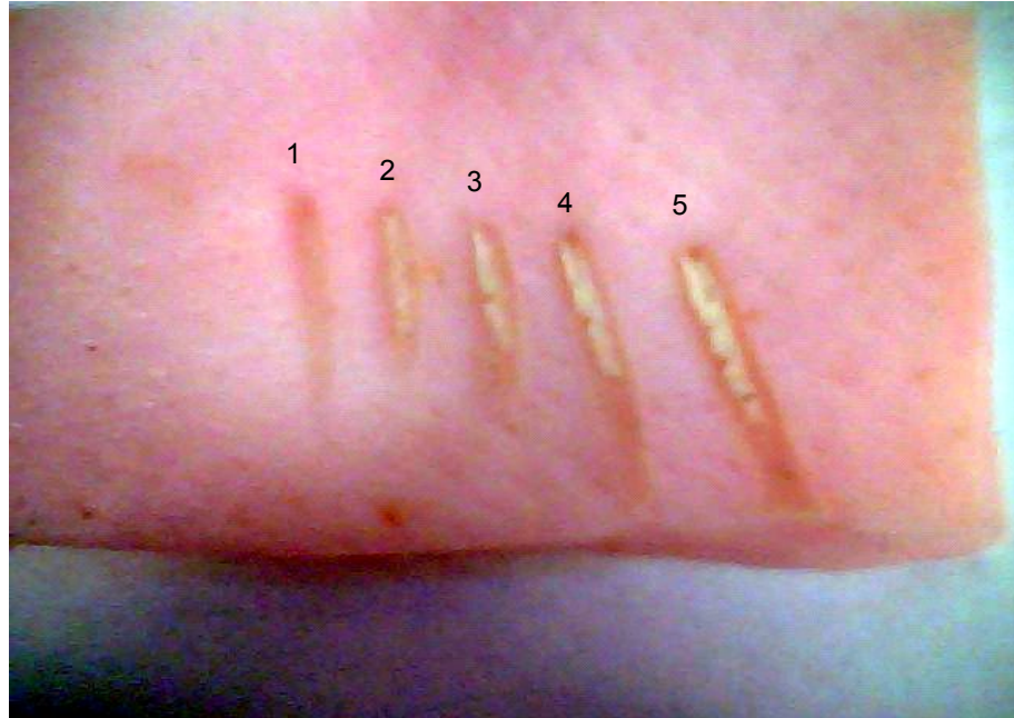
Fig. 4.8. Skin surface burns (1) 600 °F 1sec., (2) 600 °F 2sec., (3) 600 °F 3sec., (4) 600 °F 4sec., and (5) 600 °F 5sec.,
