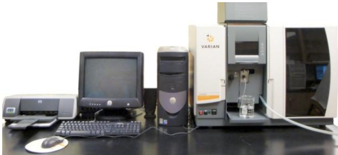
Figure 1.4: Flame atomic absorption spectrometer owned by the Department of Chemistry at Wright State University. (photo courtesy of Garrett VanNess)
