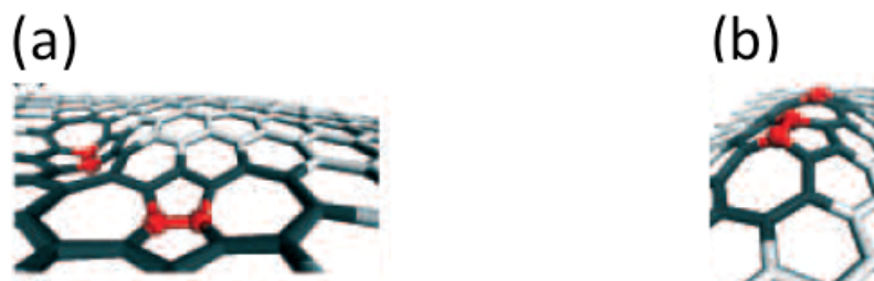
Figure 3.1.6 Nonlinear (a) and linear (b) arrangement of ISWD 30 .
