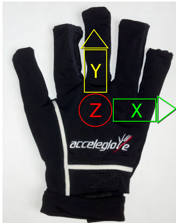
Figure 2.1: The reference axes for the AnthroTronix AcceleGlove
