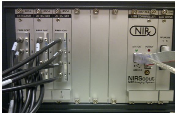
Figure 3.1: Face of the tabletop NIRScout NIRS imaging system. The dimensions of this main unit are 26 x 17 x 33 cm (WxHxL). Ports on the front, from left to right, include twelve detectors, USB output to a data acquisition computer, parallel input from a stimulus computer, and eight NIR sources.
