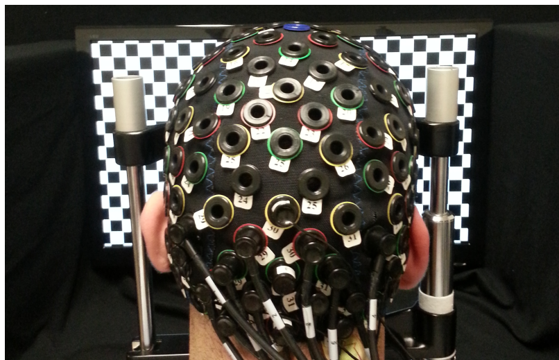
Figure 4.3: Example of the experimental setup for the visual cortex protocol (including the optode configuration), as viewed from directly behind the participant. The participant's head is supported by a chin rest, which is a fixed distance away from the stimulus display screen on which a checkerboard pattern can be observed. Five sources and twelve detectors were utilized to provide a sampling frequency of 8.929 Hz. The specific layout can be seen in Figure A.4 of Appendix A.
