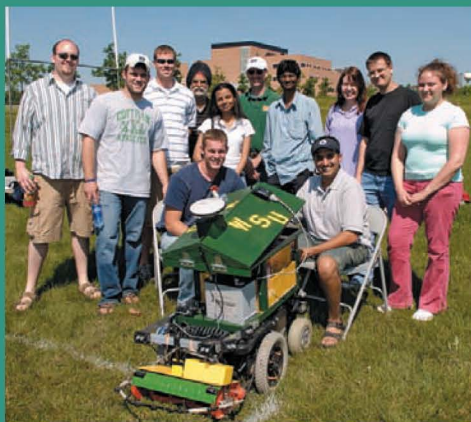
The WSU automow team created their autonomous lawn-mower by modifying an electric wheelchair.
