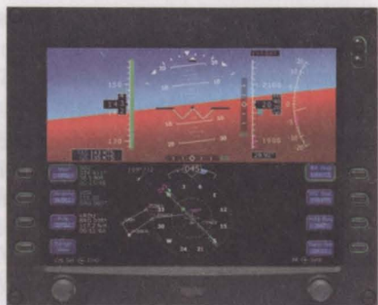
Figure 1. The Avidyne primary flight display (PFD). The same display was used for training in the flight simulator and in the transfer aircraft.
