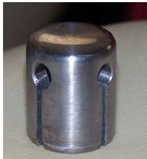
FIG. 3. Niobium cathode. The machined holes and slots on each side of the cathode allow insertion of a tool used to press the cathode into the cathode stalk, and allow the cathode base to flex for a tight fit during insertion. In this way, the cathode can be inserted without risking damage to its emitting surface.
