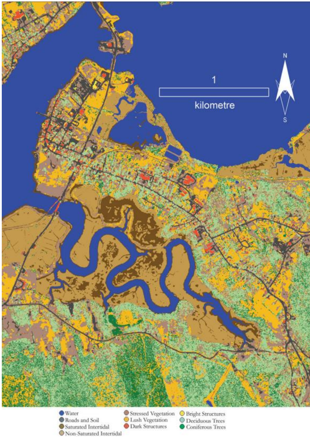
Figure 2. Terrain classification conducted using LiDAR intensity, a generated DSM, normalized height, and return number. 13
