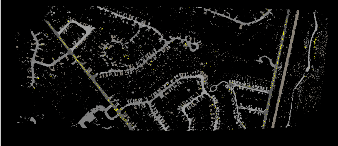
Figure 36. Demonstration of ML Classifier results with a medium probability threshold (0.50) showing spectral classes 2–5 and 11, highlighting roads, railroads and road paint.
