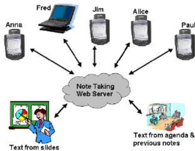
Figure 1. Notes taken by students and text extracted from related material is shared among students
