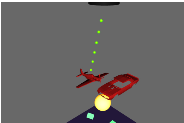
Figure 3: The second example: a scene of two colliding convex hull rigid bodies constrained using the BallJoint and MotorJoint type.
