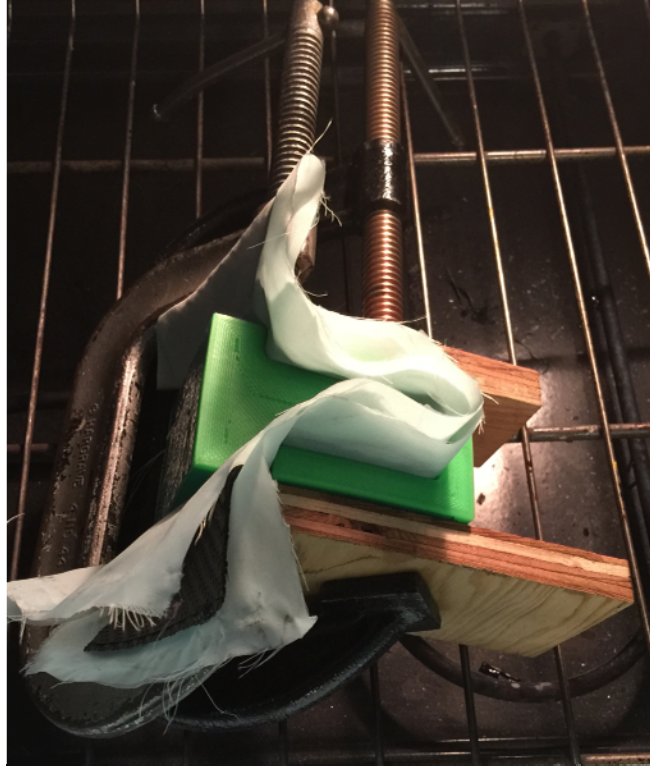
Figure 56. Molds with G-clamps and strong backs.
