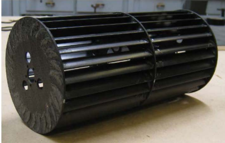
Figure 26. Complete manufactured 26-bladed rotor, from [4].
