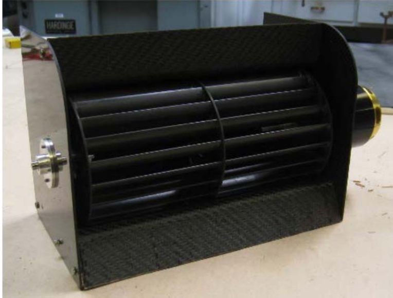
Figure 2. Carbon fiber cross-flow fan and housing unit, from [4].
