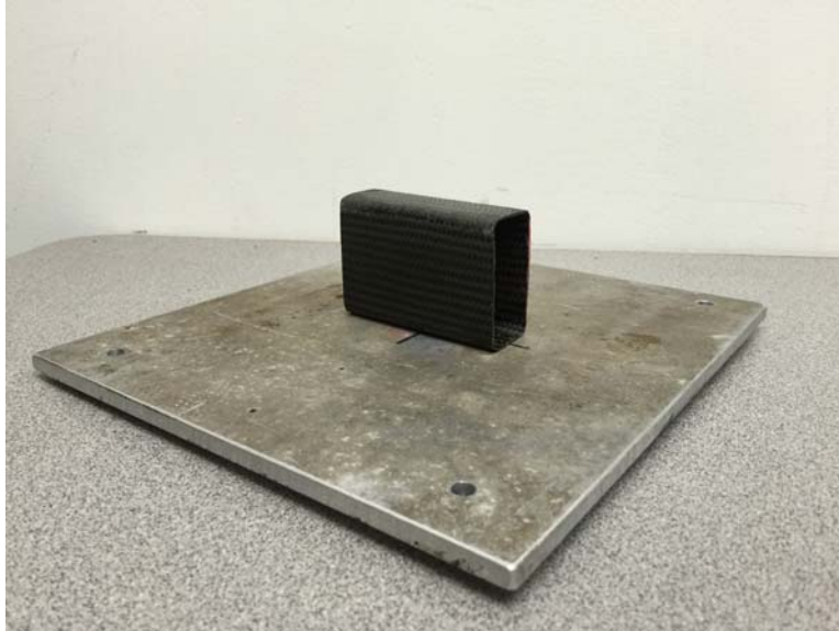
Figure 18. Tubing mold assembly used to make carbon fiber frame clamps.
