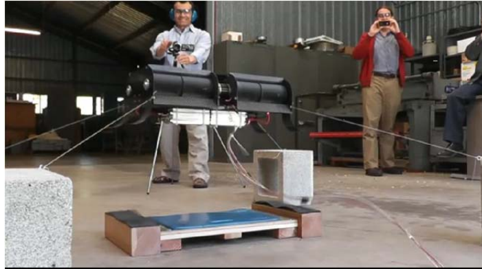
Figure 8. Airframe with four fans powered by two motors, from [2].
