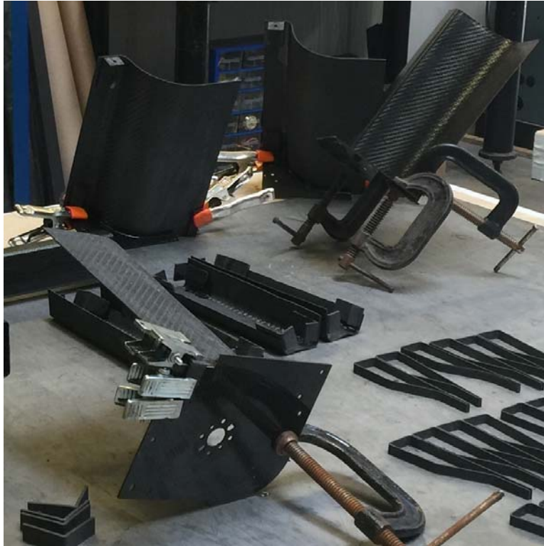
Figure 43. Fan housing epoxy process.
