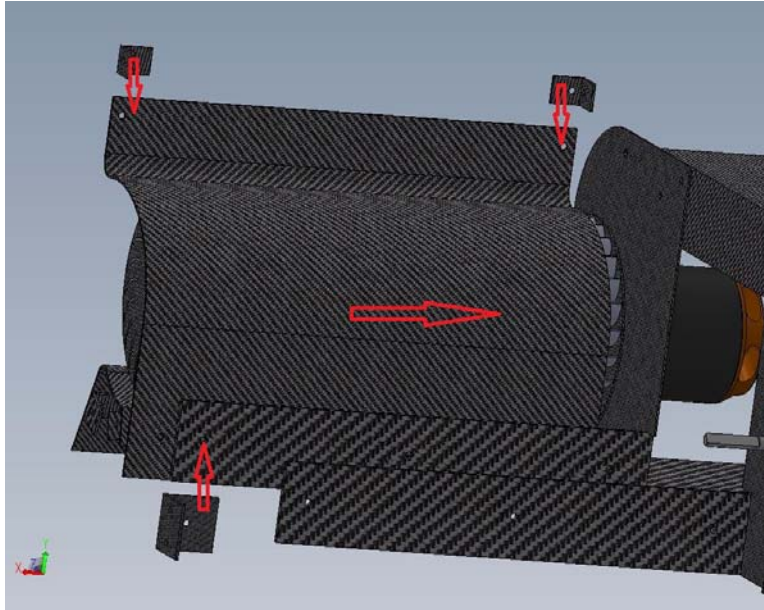
Figure 65. Intake housing to airframe foundation.
