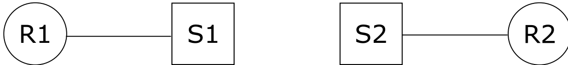
Figure 3.3: The path between the two routers after the link has been cut. The interfaces connected to the switch on each router will still be powered; each router assumes connectivity to the other until the “dead timer” expires.
