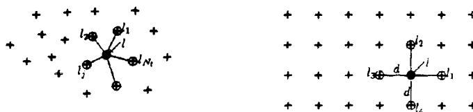
Figure 2 Part of a general grid (left) and a regular quadratic grid with grid constant d (right).
