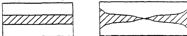
Figure 2: a) Conventional resonator b) Resonator shaped for maximum Q
