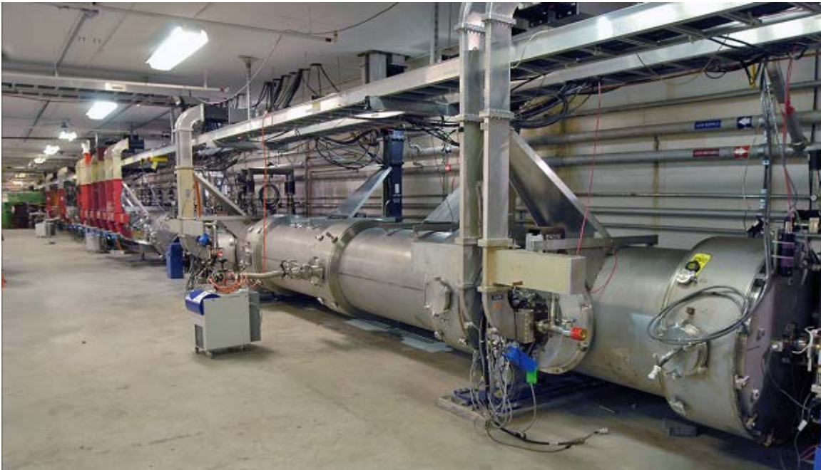
Figure 2. Free Electron Laser (from Jefferson Lab News 2006)
