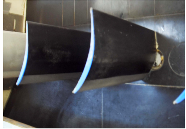
Fig. 4 Picture of roughened blades (20% suction side of the baseline blade)
