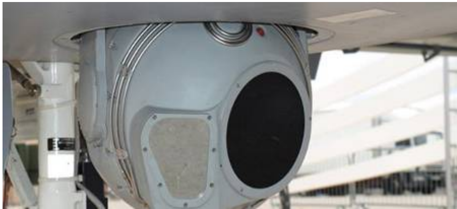
Figure 3. EO/IR payload (from Defense-Update, 2009)
