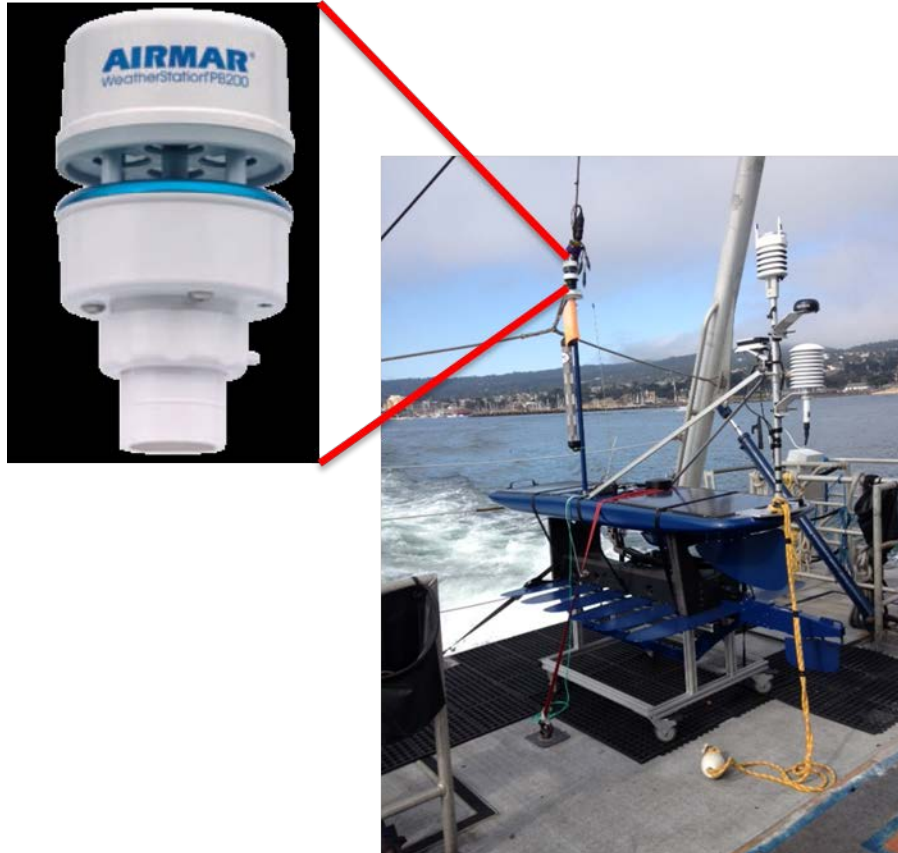
Figure 9. Airmar PB200WX weather station mounted on the SHARC.
