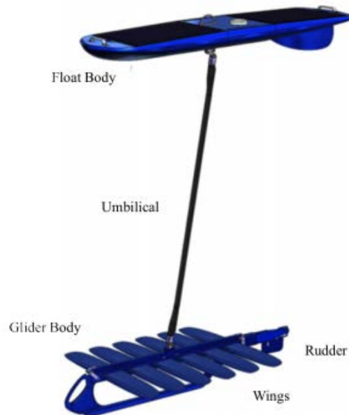
Figure 6. Illustration of main components of SHARC (from Rochholz 2010).
