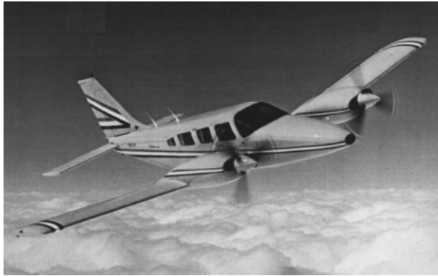
FIG. 7. Piper Seneca III light twin-engine aircraft instrumented and operated by the University of North Carolina at Chapel Hill.
