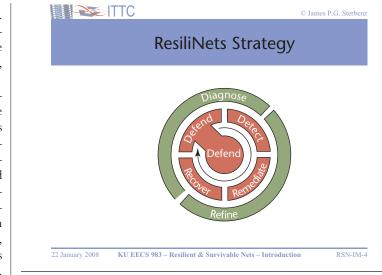
Figure 1. ResiliNets. James Sterbenz's model views resilience as a twophase process. The inner phase is a never-ending cycle of network defense, detection, remediation, and recovery. The outside phase is aimed at process improvements: diagnosing the root causes of successful attacks and refining the tools and human behavior in use.
