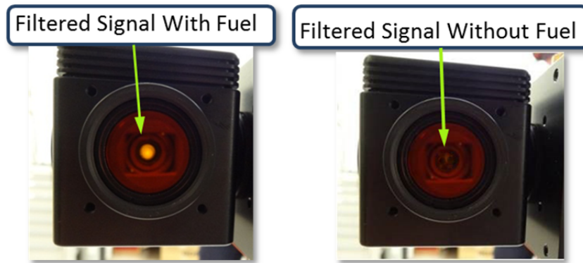
Figure 29. The left image show the fluorescence response from a jar of fuel reaching the sensor, the right image shows no response reaching the sensor when the fuel is moved away.
