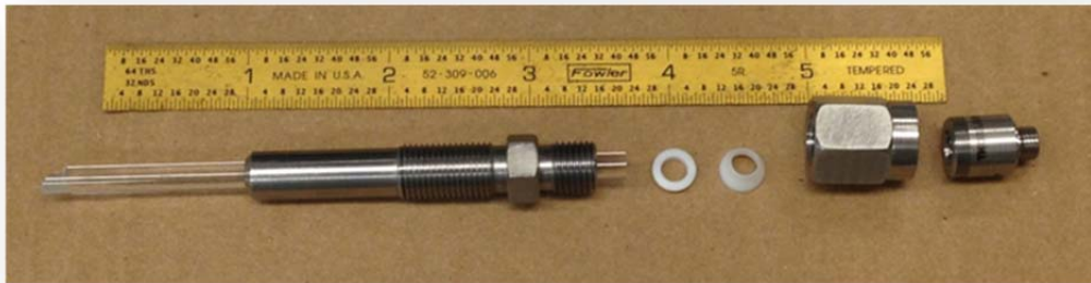
Figure 14. Sapphire rod, upper and lower rod housings with PTFE ferrules, and collimator lens.
