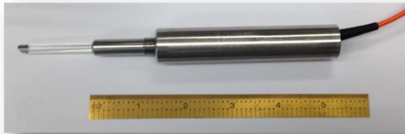
Figure 15. Complete sapphire rod assembly, sapphire rod and lower housing protruding from the sleeve.
