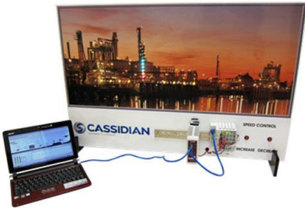
Figure 8. Tofino SCADA Security Simulator, from [16]
