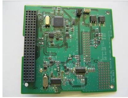
Figure 6. NPS-SCAT Beacon Board Built by Brian Tubb and Sean Fitzsimmons
