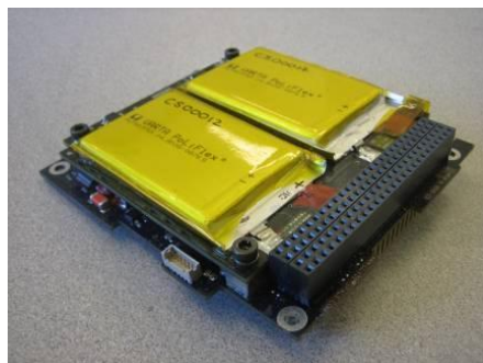
Figure 5. Clyde Space EPS and Battery
