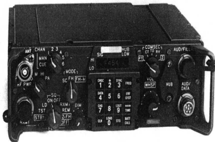
Figure IV-18. SINGGARS RT-1523 Transceiver
