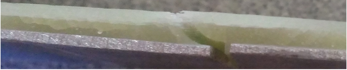
Figure 12. Side view of sample 5 showing delamination in composite
