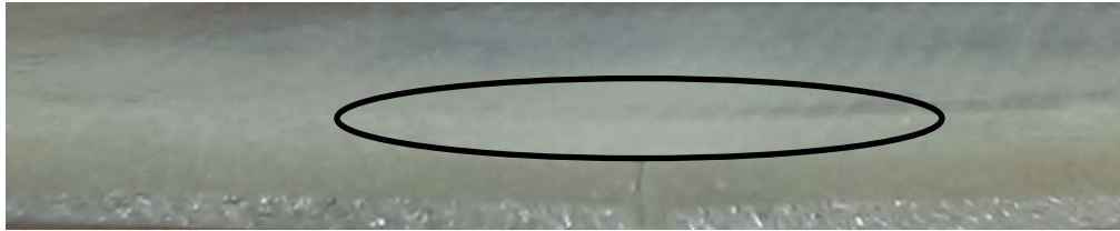
Figure 27. Sample 2 showing delamination within the composite only
