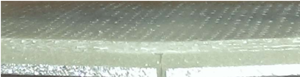
Figure 28. Sample 2 showing no delamination between layers or aluminum
