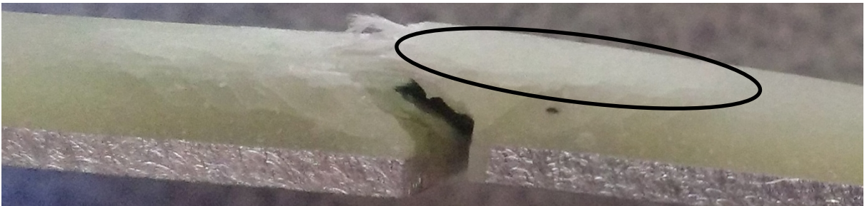
Figure 16. Side view of CNT sample 5 showing small delamination in composite
