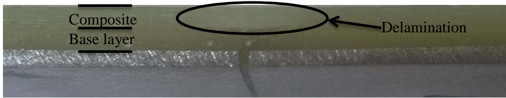
Figure 22. Sample 4 showing delamination within the composite only
