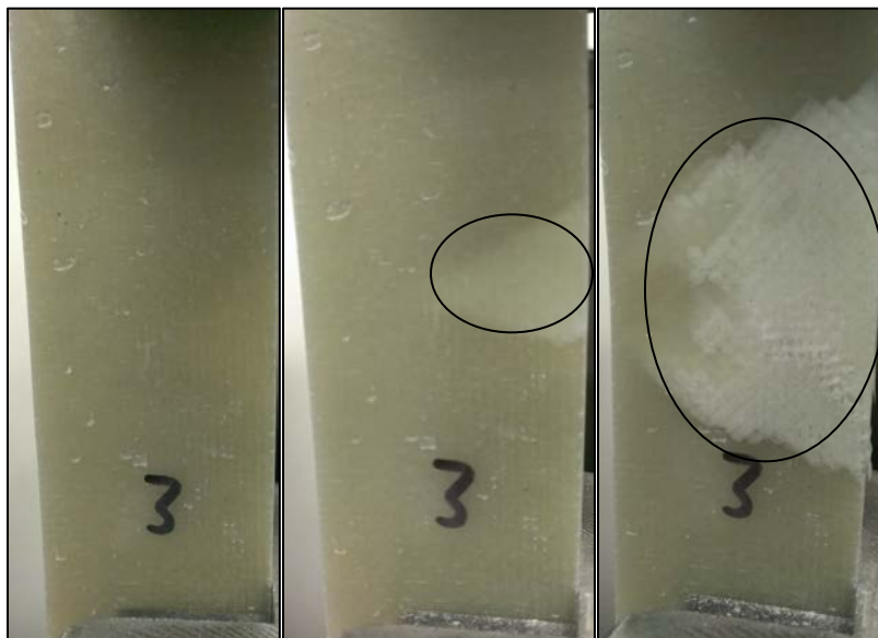
Figure 38. Full length composite sample, initially unloaded (left), initial delamination (middle), final delamination (right)
