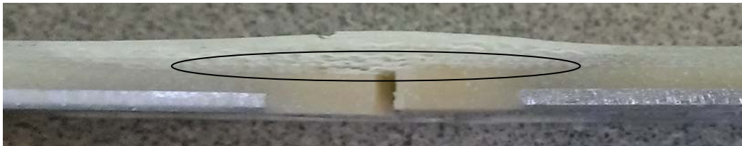
Figure 39. Full length composite sample showing delamination between the base resin layer and the composite
