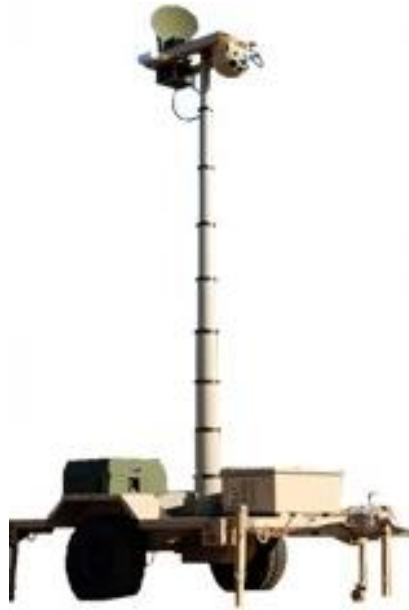
Figure 14. Trailer-mounted GBOSS system configured for operation 69
