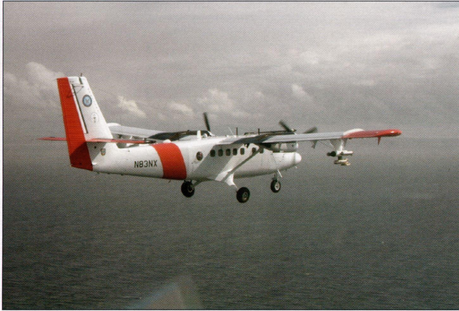
Fig. 1. The CIRPAS UV-18A Twin Otter turboprop research aircraft. This twin turboprop Short Takeoff and Landing (STOL) aircraft can cruise at low speeds for long durations over the ocean with a maximum endurance of 8 hours, maximum altitude of 7600 m, 35–80 m/s operational speed range, 200 amps of payload power, and an approximately 2400 kg useful load.
