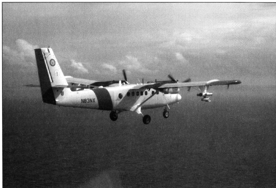
Fig. 1. The CIRPAS UV-18A Twin Otter turboprop research aircraft. This twin turboprop Short Takeoff and Landing (STOL) aircraft can cruise at low speeds for long durations over the ocean with a maximum endurance of 8 hours, maximum altitude of 7600 m, 35–80 m/s operational speed range, 200 amps of payload power, and an approximately 2400 kg useful load. Original color image appears at back of this volume.
