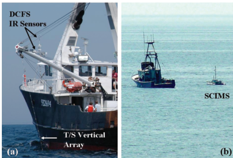
FIG. 7. (a) Instrumentation deployed on the Nobska during the 2003 IOP. Bow instrumentation included a direct covariance flux system and IR radiometers. The boom supported an array of temperature–salinity sensors for high-resolution vertical profiles. (b) Photo taken from the Air–Sea Interaction Tower at MVCO of the SCIMS catamaran accompanied by R/V Asterias during a southeasterly survey transect on 15 Aug 2003. Numerous banded surface film features (light areas) evident in the field of view were quantified by SCIMS instrumentation.
