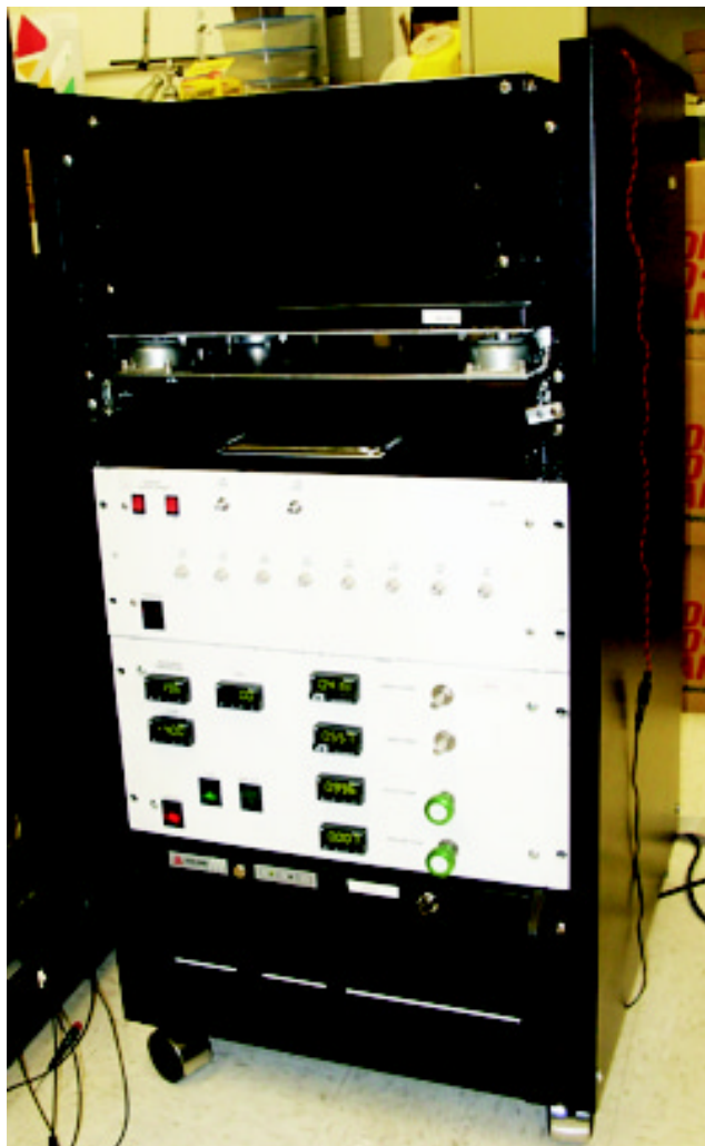
Figure 3. Picture of Cadenza mounted in a 19-inch equipment rack in our lab showing overall height of 40 inches.
