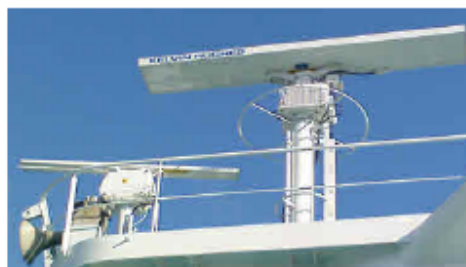
25kW Upmast X-Band and 30kW Upmast S-Band Transceivers
